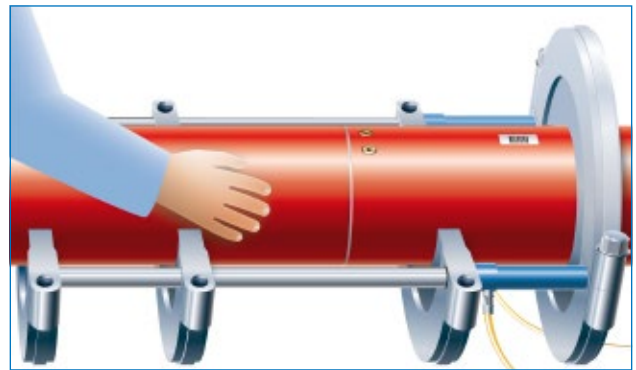
Insertion of the spigot ends into the socket has to be a priority
