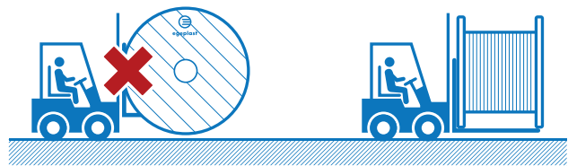
Lifting the drums only via the wooden wheels.
