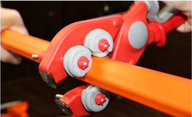
1. Notch the sheathing with the circular pliers at two spots at a distance of 60-100 cm from each other.
