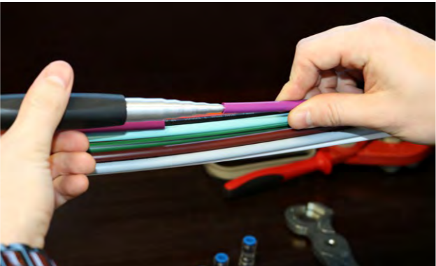
6. Reround the interfaces using the 5/20 tool.
