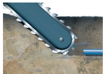
Fig 1-2: Schematic diagram Milling procedure
