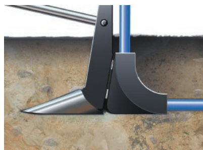
Fig 1-1: Schematic diagram Ploughing procedure
