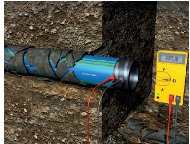
Fig. 25: Continuity check as evidence of lack of damage to the new pipeline
