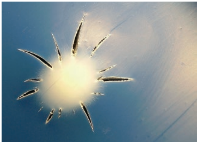
Fig. 19: Stress crack on the inside of the pipe caused by point load and incorrect choice of material (source: HESSEL technical engineering)
