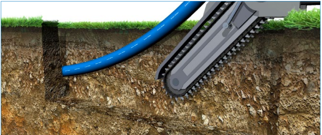
Fig. 6: Since excavated soil is used as backfill material in the milling method it is recommended that pipe systems with integrated protective layers be used.
