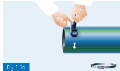
Fig 1-16 Removal of the protective layer with suitable peeling tools
