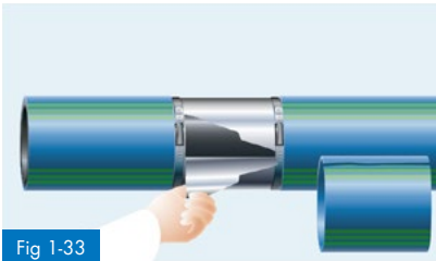
Fig 1-33 Removal of the aluminium barrier by means of a hose clip
