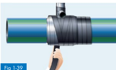
Fig 1-39 Wrapping the tapping fitting with Densolen Tape AS 40
