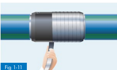
Fig 1-11 Wrapping of the welded fittings with aluminium adhesive tape
