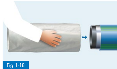
Fig 1-18 Mount shrinking sleeve prior to manufacture of the pipe joint, do not remove the protective foil
