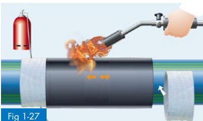
Fig 1-27 Shrinking of the sleeve by means of a soft gas flame
