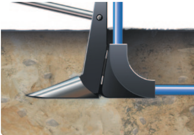
Fig 2-4: When using the ploughing installation method, the use of pipelines with integrated protective layers is recommended.
