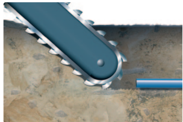
Fig 2-5: Since excavated soil is used as backfill material in the milling method it is recommended that pipe systems with integrated protective layers be used.
