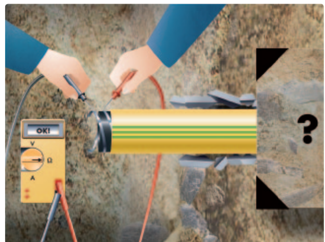
Fig 2-27: Continuity check as evidence of lack of damage to the new pipeline
