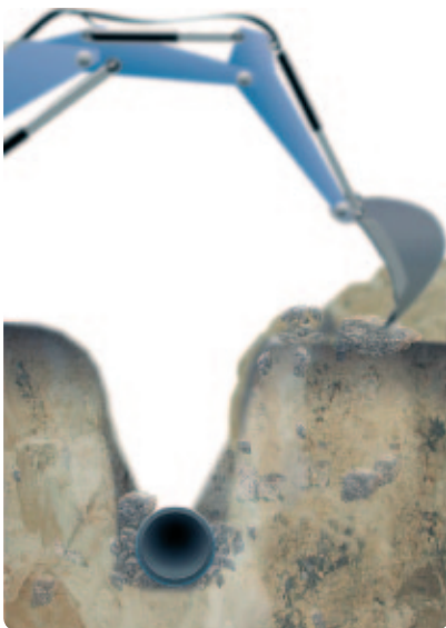
Fig 2-3: When installation is not executed in a sandbed, pipes with integrated protective layers are recommended to be used.
