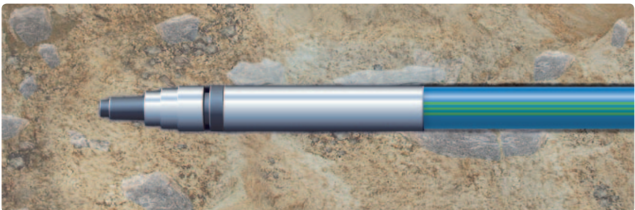
Fig 2-6: It is necessary to use pipelines with additional protective layers because installation using impact moles can damage the pipeline that has been injected.
