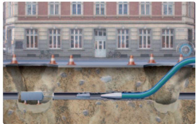
Fig 2-11: Static Pipe bursting
