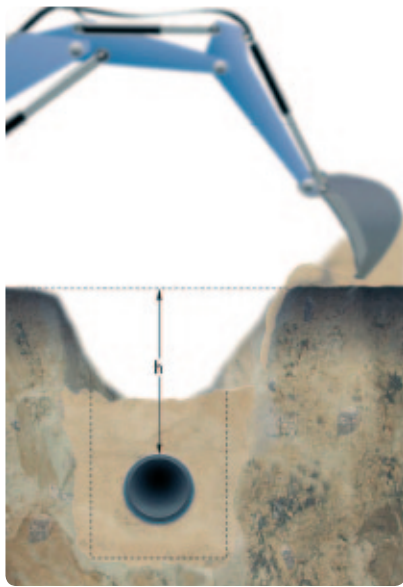
Fig 2-2: Standard pipes are installed in a sand bed.
