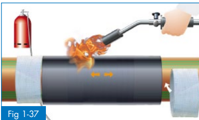
Fig 1-37 Attaching the heat shield and applying the heat shrink product
