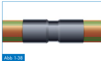
Abb 1-38 Welded joint protected by the heat shrink product
