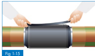
Fig 1-15 Sealing the contact plugs
