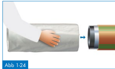
Abb 1-24 Mount shrinking sleeve prior to welding the pipe, do not remove the protective foil
