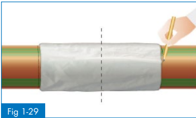
Fig 1-29 Positioning of the shrinking sleeve
