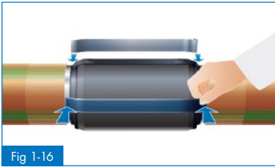
Fig 1-16 Applying of two aluminium adhesive tapes
