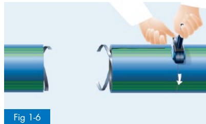
Fig 1-6 Removal of the protective layer with the egeplast M10 / M10 maxi peeling tool
