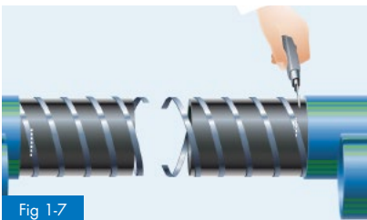
Fig 1-7 Cutting back of the conductive strips; 20 mm minimum must remain on the pipe for subsequent processing
