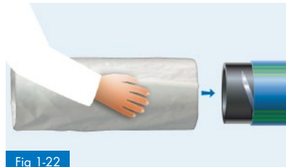
Fig 1-22 Mount shrinking sleeve prior to manufacture of the pipe joint, do not remove the protective foil
