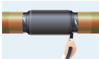
② Sealing of the ring gap between the electrofusion coupler and the pipe with filling adhesive
