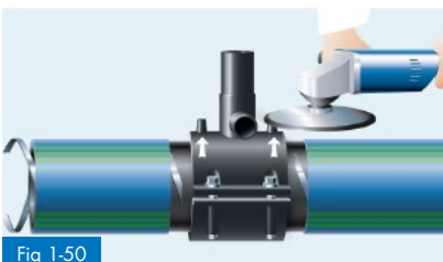
Fig 1-50 Removal of the contact plugs with a suitable tool
