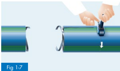
Fig 1-7 Removal of the protective layer with the egeplast M10 / M10 maxi peeling tool
