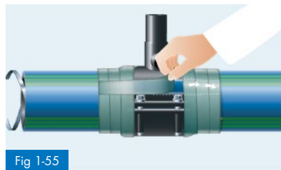
Fig 1-55 Waterproof insulation of the electrical joint
