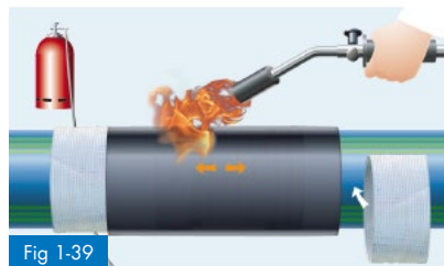
Fig 1-39 Shrinking by using a soft gas flame
