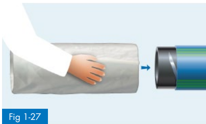
Fig 1-27 Mount shrinking sleeve prior to manufacture of the pipe joint, do not remove the protective foil
