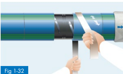
Fig 1-32 Roughen the shrink area of the sleeve radially with the emery cloth.
