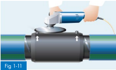
Fig 1-11 Removing the contact plugs
