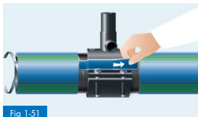
Fig 1-51 Restoring and fixing of electrical connection
