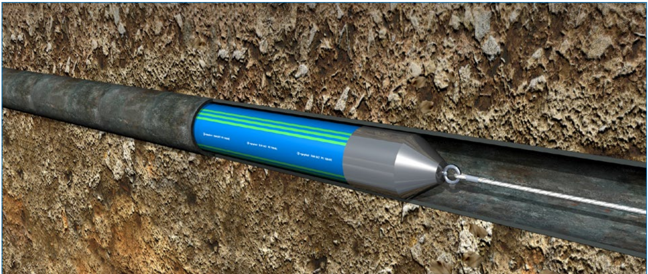
Fig. 8: The use of pipelines with additional protective layers is necessary because the new pipeline may become damaged during the relining process.
