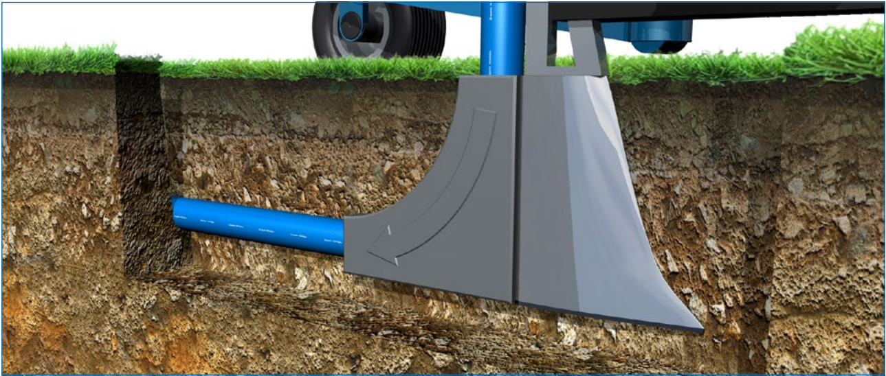
Fig. 5: When using the ploughing method, the use of pipelines with integrated protective layers is recommended.
