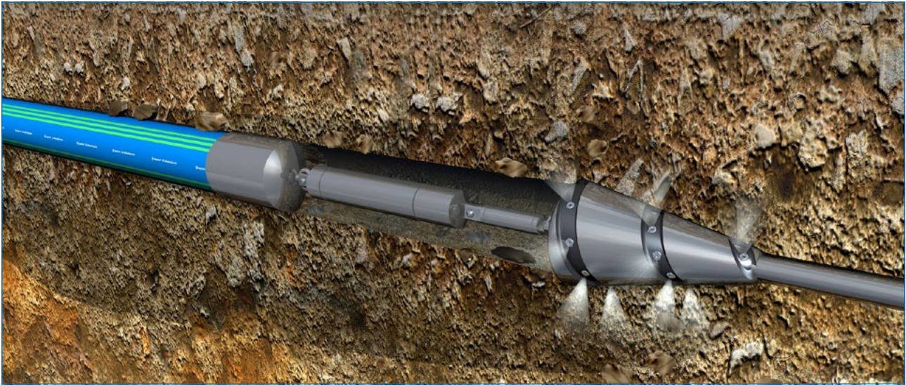
Fig. 9: The use of pipelines with additional protective layers is necessary because the new pipeline may become damaged during installation using the HDD method.
