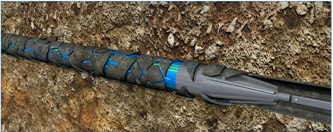
Fig. 10: The use of pipelines with additional protective layers is required because the new pipeline may become damaged during installation using the pipe bursting method.
