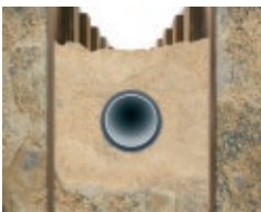
open trench installation in sandbed
